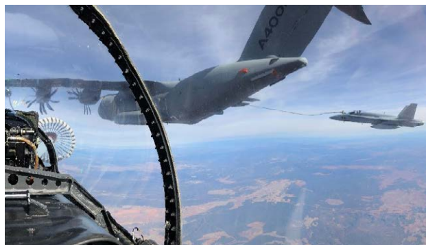
Execution of AAR through the probe-and-drogue system.
