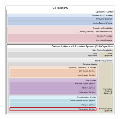
The Transmission Services cover the physical layer (also referred to as media layer or air-interface in wireless/satellite (SATCOM) communications) supporting Transport Services, as well as Communications Access Services. Support for the latter is relevant to personal communications systems, in which the User Appliances directly connect to the transmission element without any transport elements in between.
