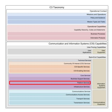
The Platform Services provide a foundation to implement services in a loosely coupled environment, where flexible and agile service orchestration is a requirement. They offer generic building blocks for implementation (e.g. discovery, message busses, orchestration, information abstraction and access, etc.) and can be used as a capability integration platform in a heterogeneous service-provisioning ecosystem.
