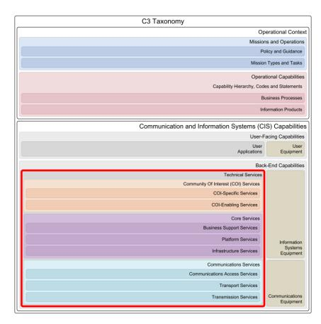
The "Technical Services" taxonomy layer represents the collection of services with requirements for software and hardware functionalities that can be reused for different purposes, together with the policies that should control their usage. These requirements are derived from the operational needs expressed by the collection of User-Facing Capabilities. Inherently, the Technical Services must support all Mission Types and Operational Capabilities.
