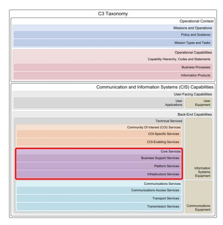
The Core Services provide generic, Community of Interest (COI)-independent, technical functionality to implement service-based environments using infrastructure, architectural and enabling building blocks. Core Services provide these building blocks so that these generic, common capabilities do not have to be implemented by individual applications or other services.
