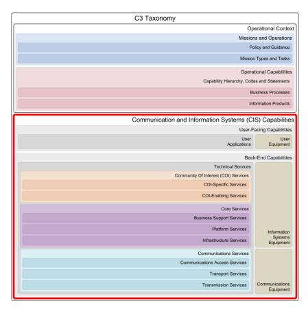
The C3 Taxonomy layer for the "Communication and Information System (CIS) Capabilities" represents the logical components of the capabilities required to meet NATO's information system and communication needs in support of Missions and Operations.
