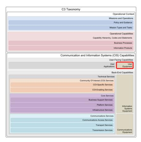
The "User Equipment" taxonomy layer represents the collection of equipment that is involved in the physical interface between users and User Applications. This equipment is deployed in various environments, which will have implications for ergonomics, form factors, physical and electrical specifications, and more.
