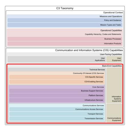
The "Back-End Capabilities" layer in the C3 Taxonomy represents the catalogue of services and equipment that is required to enable User-Facing Capabilities. The catalogue expresses the requirements for data processing and communications.
