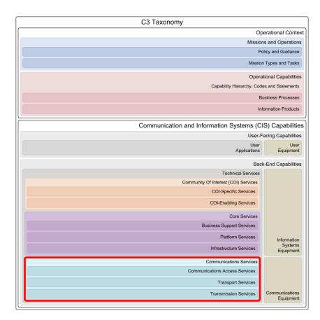
The Communications Services interconnect systems and mechanisms for the opaque transfer of selected data between or among access points, in accordance with agreed quality parameters and without change in the form or content of the data as sent and received.
