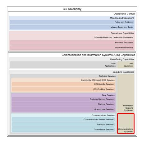
The "Communications Equipment" taxonomy layer represents the collection of equipment that is involved in the transfer of data that make up the networking and physical communications links for the enabling of Communications Services.
