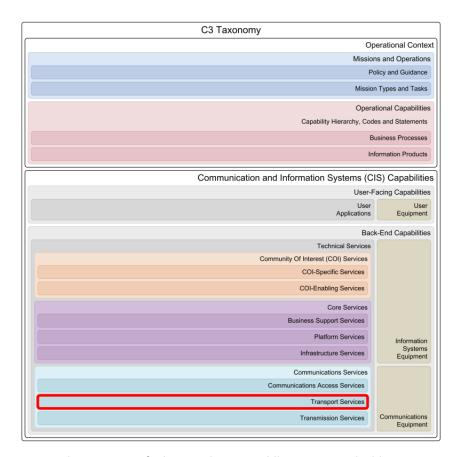
The Transport Services correspond to resource-facing services, providing metro and wide-area connectivity to the Communications Access Services that operate at the edges of the network. In that role, Transport Services interact with the Transmission Services using them as the physical layer fabric supporting the transfer of data over a variety of transmission bearers as and where needed.
