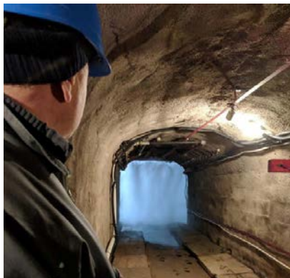
A water mist curtain helps to confine the fuel cloud explosions, as demonstrated at the test site in Tbilisi
