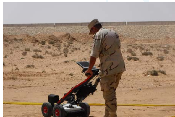
An Egyptian military engineer is testing a Ground Penetrating Radar mine detector
