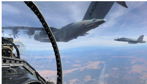
Execution of AAR through the probe-and-drogue system.
