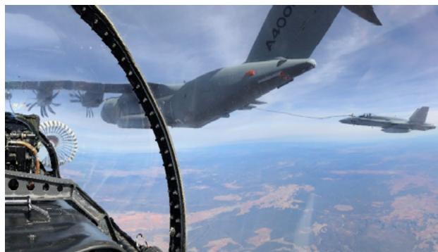
Execution of AAR through the probe-and-drogue system.
