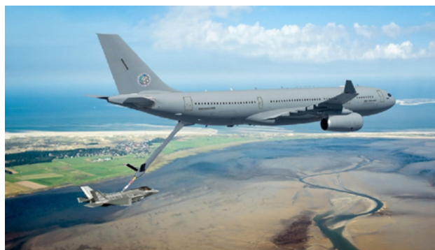
Airbus A330 Multi Role Tanker Transport aircraft executing AAR through the boom system.
