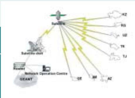
→ The SILK Network configuration consists of satellite dishes and network equipment in each of the eight participating countries, a central distribution point (hub) with a dish and network equipment in Western Europe, a contract with a satellite vendor and Internet access. A common satellite beam will connect the academic and educational communities of the eight countries to the Internet.
