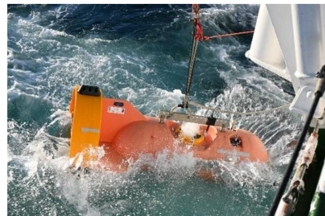
Figure 9: ACO24 sea trial, July 2024: recovery by NRV Alliance of the top float of an underwater mooring deployed for the NATO Arctic Climate Observatory in July 2023.
