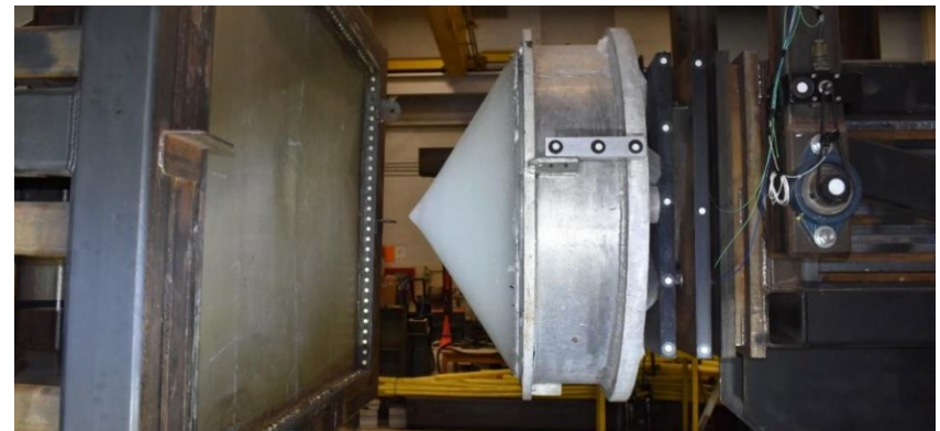
Figure 18: Lab-grown, one-metre diameter ice cone (right) and steel warship hull specimen (left) fixed into an ice impact apparatus before testing [Photo credit: Prof. Bruce Quinton, Memorial University of Newfoundland, used with permission].
