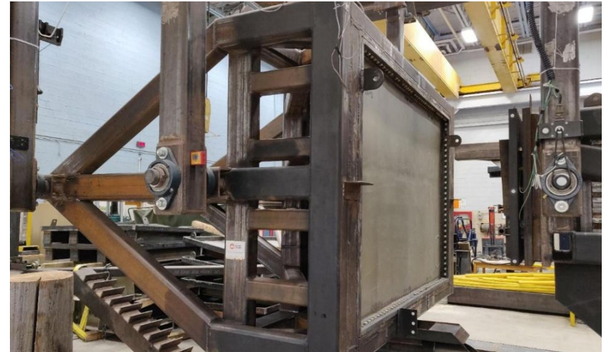
Figure 17: Actual steel hull plating that was removed from the decommissioned Canadian warship, ex-HMCS Iroquois, and bolted into a testing frame for ship-ice impact experiments [Photo credit: Prof. Bruce Quinton, Memorial University of Newfoundland, used with permission].
