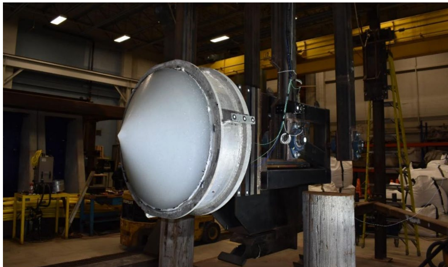
Figure 16: Cone-shaped ice specimen grown in the laboratory for ship-ice impact experiments [Photo credit: Prof. Bruce Quinton, Memorial University of Newfoundland, used with permission].
