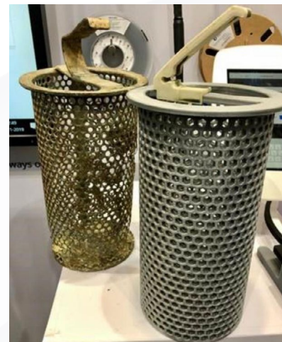
Figure 32: OEM filter (left) versus the polylactic acid printed filter (right). Photo: Jonas Leander.
