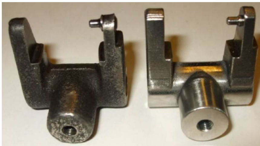
Figure 31: Engine speed governor. Original part (left) and additively manufactured part (right).
