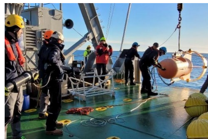
Figure 10: ACO24 sea trial, July 2024: recovery by NRV Alliance of the top float of an underwater mooring deployed for the NATO Arctic Climate Observatory in July 2023.
