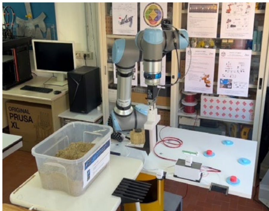
Programming of the robot's manoeuvres for mine detection and extraction
