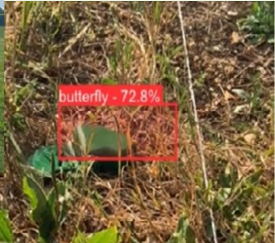
Screenshot showing PFM-1 "butterfly" scatter-able mine detected with 72.8% confidence by AI app.
