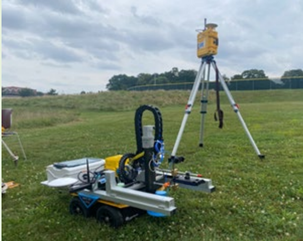
Robot with holographic radar scanning system and shared GPS/communications base station in background.
