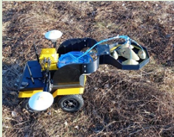
Robot with cm-accuracy GPS (white) and 1TX-4Rcv impulse GPR (gold).
