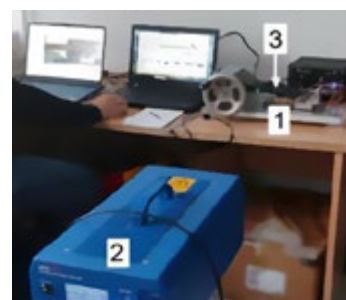
The experimental setup used to study the influence of the dynamic mechanical properties of materials on the structural vibrations of samples made from acoustic materials developed within the project.
