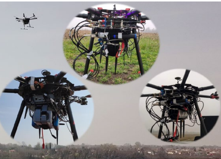
Figure 16 - Different receivers and antennas fitted to UAVs in the context of the SPS MYP "Counter-terror".
