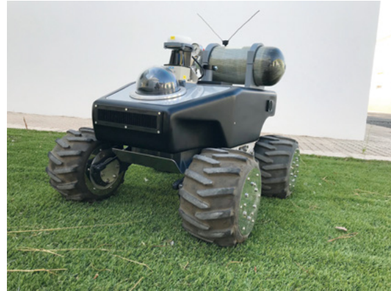
Figure 26 – UGV with hydrogen storage system developed in the framework of SPS MYP 'Improving Efficiency and Operational Range in Unmanned Vehicles using Fuel Cells'.
