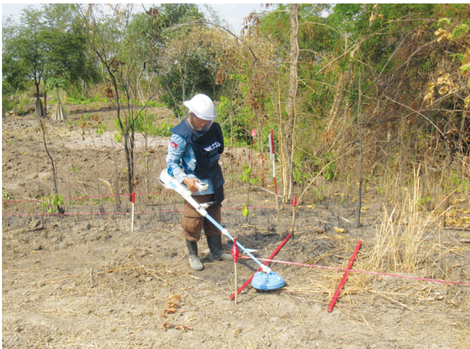
Figure 43 – Field demonstration of the ALIS detector.
