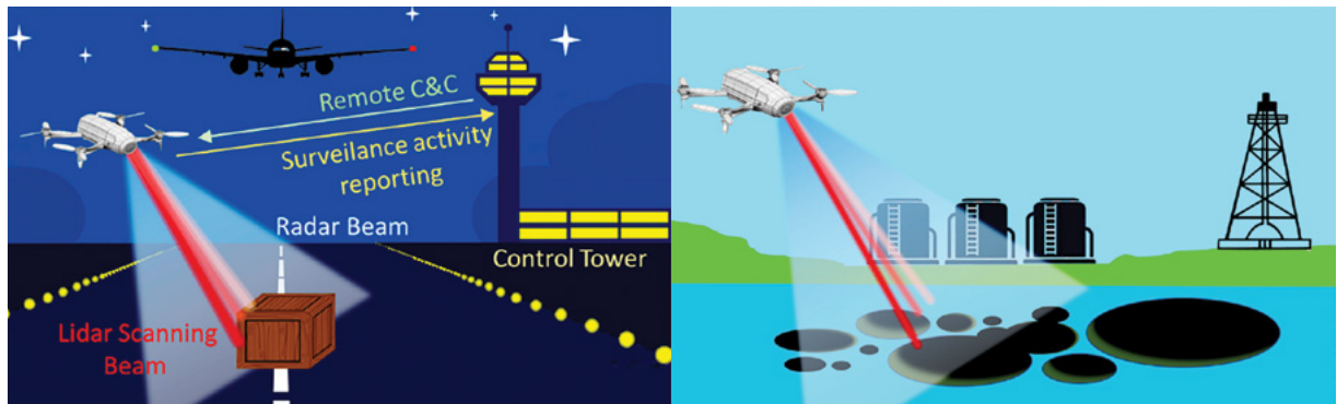
Figure 16 - Two possible scenarios of application of the proposed CLARIFIER integrated radar-lidar system. Up: Detection of (intentional or unintentional) obstacles in sensible infrastructures, e.g. airport runways. Down: Early oil spill detection in docks.
