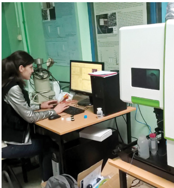
Figure 34 - Young researcher from the Institute of multidisciplinary research, while using ICP-OES equipment to investigate the leaching of hazardous elements from alkali-activated matrices.
