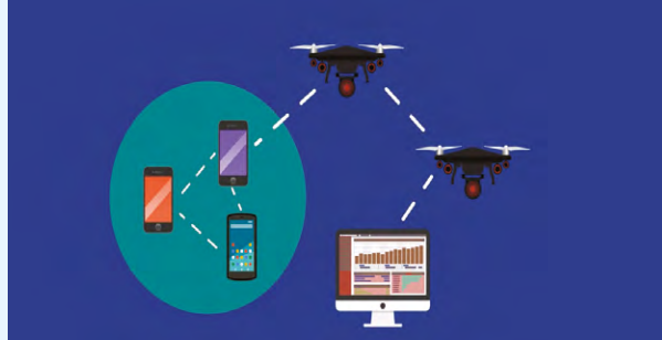
Figure 35 Model of a prototype system using WiFi-Direct enabled handsets, UAVs, and a command control center
