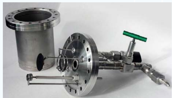
Detail of a chamber for purification and purity control developed by the project team. © NATO
