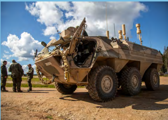
German CG20+ mobile counter-UAS system during exercise Baltic Trust 25. Latvia, August 2025.
