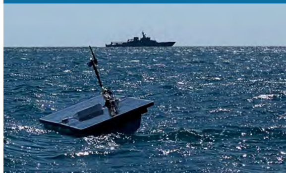
Online Oceans Solar Scout, a long-endurance autonomous ocean drone taking part in REPMUS 25. Portugal, September 2025.
