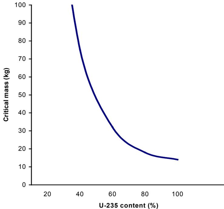
*Figure A4. Critical mass of uranium metal in the form of spheres enclosed in thick neutron reflectors of natural uranium, as function of enrichment levels.<sup>177</sup>*
