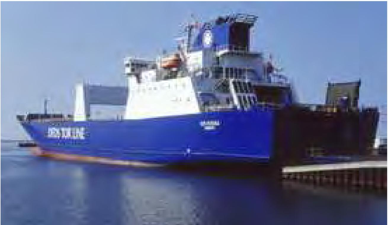
This multinational consortium finances the charter of up to 11 special “roll-on/roll-off” ships (commonly, Ro/Ro; so called because equipment can be driven onto and off of the ships via special doors and ramps into the hold). The consortium includes Belgium, Canada, Denmark, Germany, Hungary, Lithuania, the Netherlands, Norway, Portugal, Slovenia and the United Kingdom.
