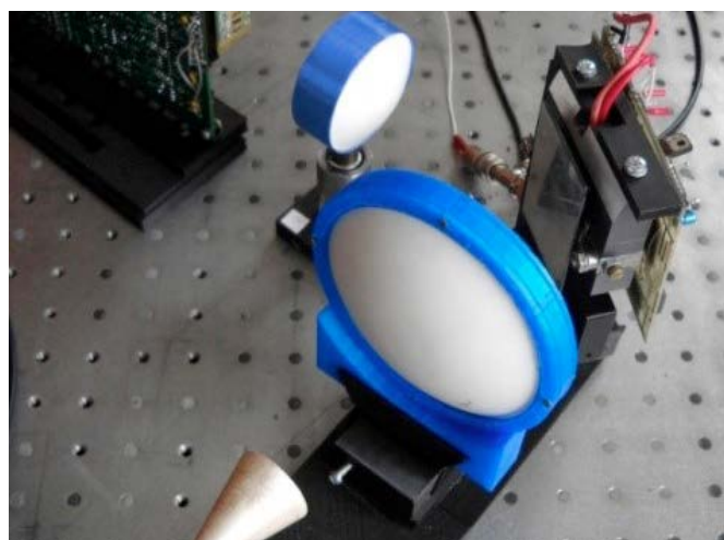
THz active optical system with aspheric lenses and scanning mirror for obtaining THz images
